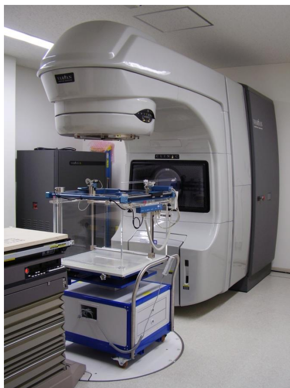
Fig. 2 Electron linear accelerator available for education and research not for clinical use
