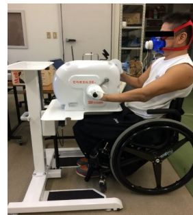
Breath gas analysis using upper body ergometer
