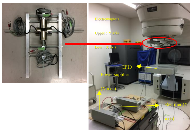
Development of image acquisition device by bending of electron beam using electromagnets
