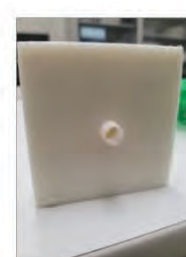
Development of new blood vessel phantom
