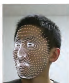
Automated patient authentication by face authentication using Kinect
